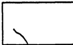
Frame cracks, caused by settling or the result of poor or old construction.
