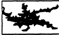
Big, jagged hole typical damage from a rock or brick.
