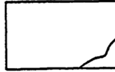
Corner cracks, resulting from strain caused by settling or settling of building.
